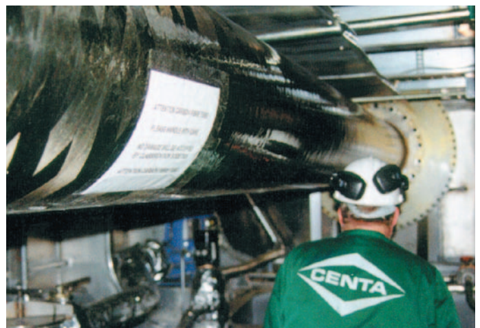
CENTADISC carbon fibre shaft in »Jumbo Cat«.
