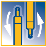
Installation position any as required Einbaulage beliebig
